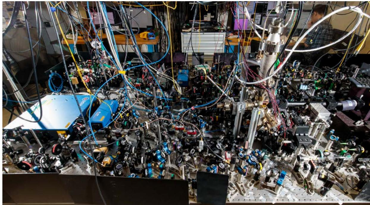
To perform experiments in continuous variable quantum computing, the group uses this entire setup. It occupies a table measuring 4m x 1.5m. In total, there are about 400 to 500 optical elements such as mirrors and lenses.
