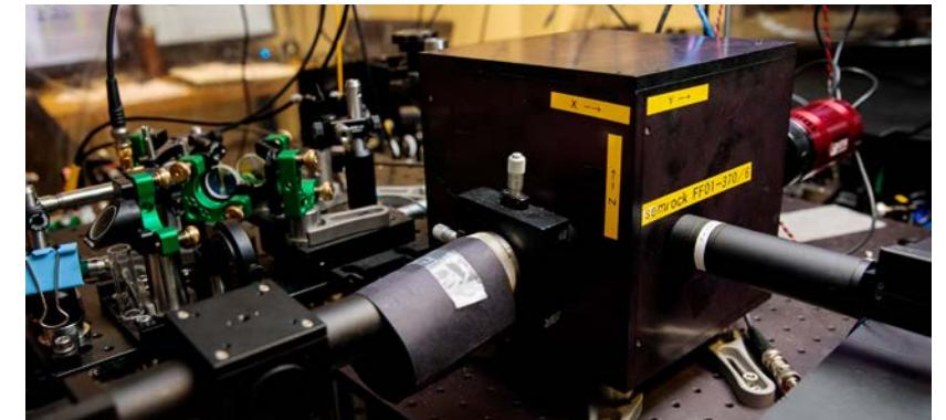
These unassuming boxes act as eyes for the researchers. The ions are too tiny and dim for humans to see directly. Instead, a photomultiplier tube and camera catch light emitted from the ions to create a digital image.
