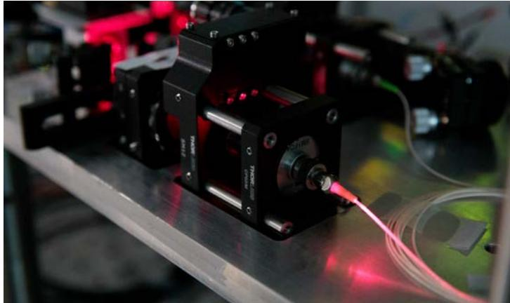
Photo: The team designed and built a quantum light source that creates entangled particles of light at wavelengths well suited to commercial optical fibre. They have wavelengths around 1316 nm, falling within the telecoms O-band.
