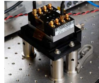
The group is making upgrades to their experiment, including adding an acousto-optic modulator with eight channels. This can direct eight laser beams, so the group will be able to control eight ions simultaneously. The team’s old modulator only had a single channel.
