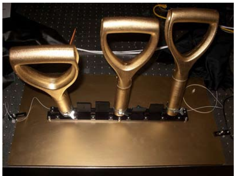
Golden Handles. Participants would use these controls of the polariser settings to try to achieve the maximal violation of Bell's Inequalities.
